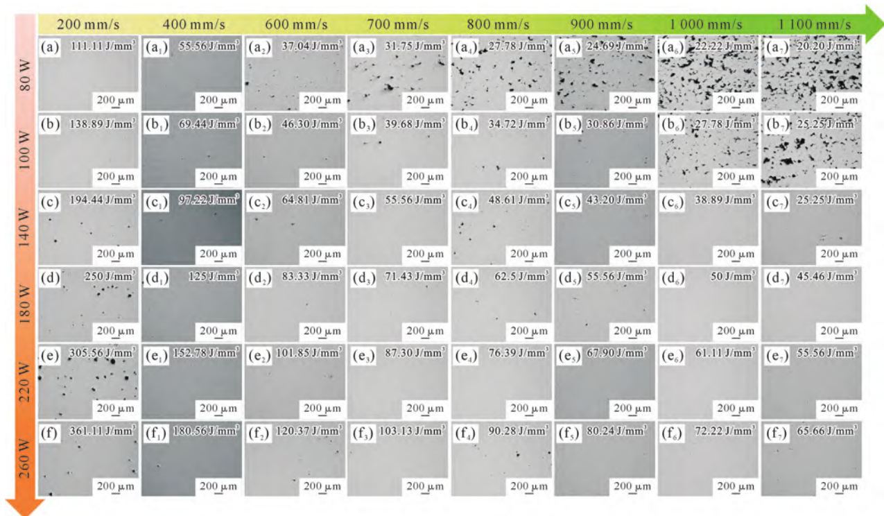
图 3 不同工艺参数 SLM 制备 Ti-22Al-25Nb 合金的光学显微组织:(a~a 7 ) 80 W, 200~1 100 mm/s; (b~b 7 ) 100 W, 200~1 100 mm/s; (c~c 7 ) 140 W, 200~1 100 mm/s; (d~d 7 ) 180 W, 200~1 100 mm/s; (e~e 7 ) 220 W, 200~1 100 mm/s; (f~f 7 ) 260 W, 200~1 100 mm/s Fig.3 Optical microstructures of Ti-22Al-25Nb alloys fabricated by SLM with different processing parameters: (a~a 7 ) 80 W, 200~1 100 mm/s; (b~b 7 ) 100 W, 200~1 100 mm/s; (c~c 7 ) 140 W, 200~1 100 mm/s; (d~d 7 ) 180 W, 200~1 100 mm/s; (e~e 7 ) 220 W, 200~1 100 mm/s; (f~f 7 ) 260 W, 200~1 100 mm/s
