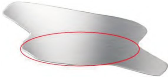
图3 叶片缘板及取样位置 Fig.3 Blade edge plate and sampling location
