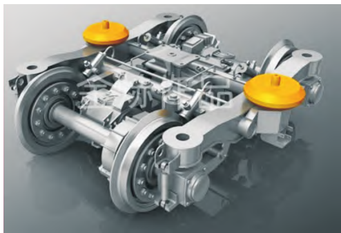
图4 轻量化转向架 Fig.4 Lightweight bogie
