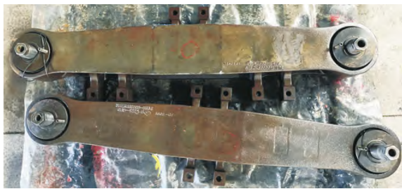
图3 ADI悬挂梁 Fig.3 ADI suspension beam
