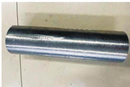
图1 K465 铸造合金母合金 Fig.1 Master alloy of the K465 cast alloy
