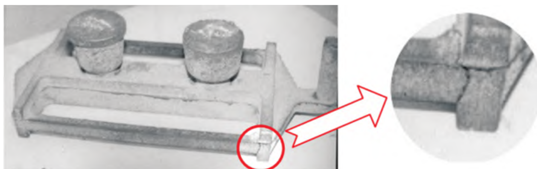
图 18 实际铸造中栅形应力框架出现的热裂缺陷 [20] Fig.18 Actual hot crack defects in the grid-shaped stress framework [20]
