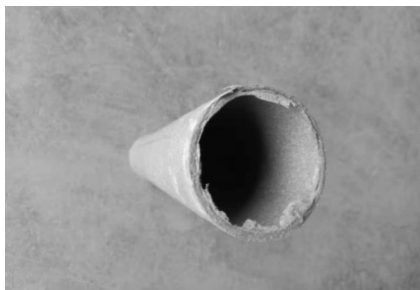
图6 毛边径向生长 Fig.6 Radial growth of burr
