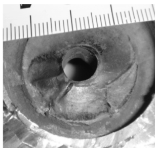
(c)断裂套管断口(另一侧)形貌
