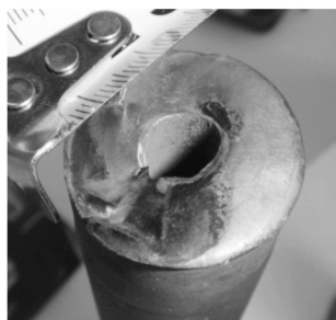
(b)断裂套管断口(一侧)形貌
