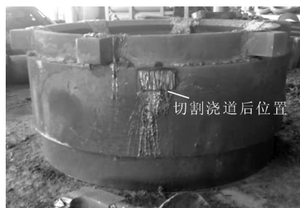
图 12 铸件外表无缺陷 Fig.12 No defects casting appearance
