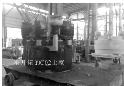
图 11 铸件出箱 Fig.11 Casting cleaning
