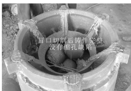
图 13 冒口补缩良好 Fig.13 Riser feeding effect
