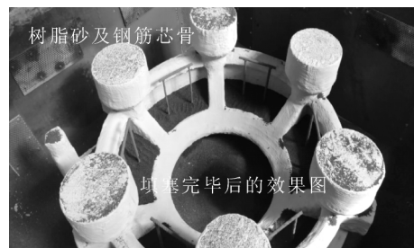
图8 填塞树脂砂并插入钢筋芯骨 Fig.8 Filling resin sand and inserting steel core bone
