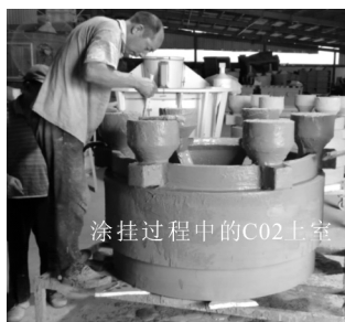
图4 手工涂挂涂料 Fig.4 Painting by hand
