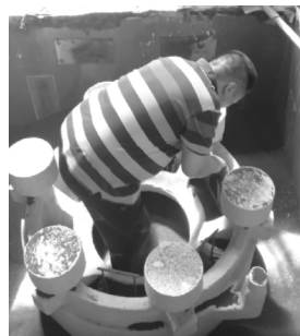
图7 盲孔填塞树脂砂 Fig.7 Blind hole filling resin sand
