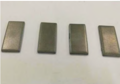
图 2 不同时间喷丸后的样品 Fig.2 Samples after shot peening at different time
