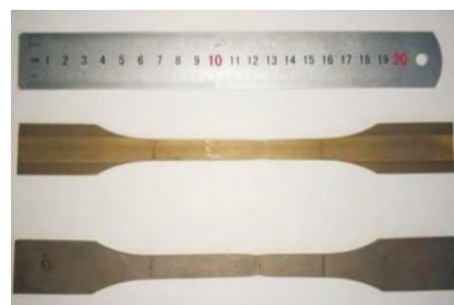
图5 室温拉伸破坏试样照片 Fig.5 Photograph of damaged specimens drawn at room temperature
