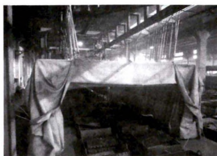
图2 可伸缩全包围式耐高温集气罩 Fig.2 Gas trap hood with high temperature resistance surrounded of retractable type
