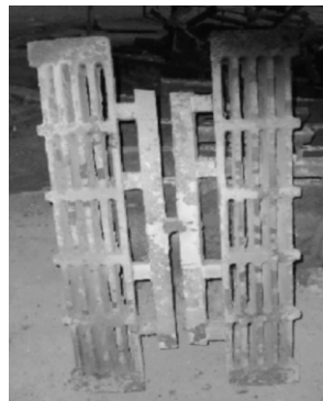
图 1 双横浇道 Fig.1 Double runner
