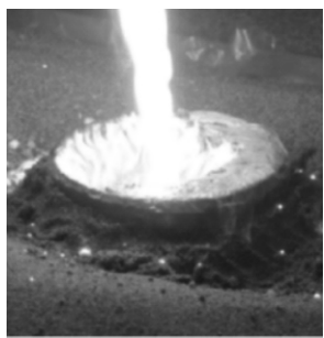
图12 钢液到处泡沫液化(三) Fig.12 The molten steel liquefied by foam (III)
