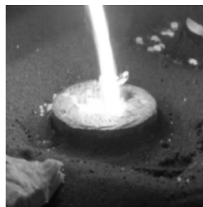
图10 钢液到处泡沫液化(一) Fig.10 The molten steel liquefied by foam (I)
