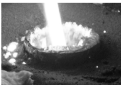
图13 钢液到处泡沫液化(四) Fig.13 The molten steel liquefied by foam (IV)
