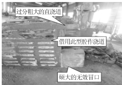
图 2 不成比例的浇道和冒口 Fig.2 A disproportionate number of gates and risers
