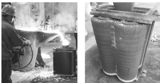
图 2 浇注过程中及浇注后砂型宏观形貌 Fig.2 Macro-morphology of sand mold during and after casting
