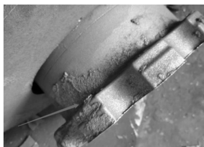
图 6 制动盘铸件粘砂缺陷 Fig.6 Sand sticking defects of brake disc casting
