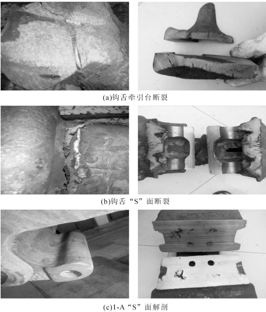
图 3 钩舌 1 断裂部位及形貌 Fig.3 Position and images of break 1
