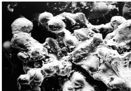
图3 缺陷位置扫描组织 ×500 Fig.3 SEM image of defects
