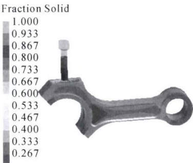
图 4 某一时刻的固相分数分布 Fig.4 Solid distribution at a certain time
