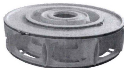
图4 大型机匣增材制造蜡模 Fig.4 Mainframe casting additive manufacturing wax mold
