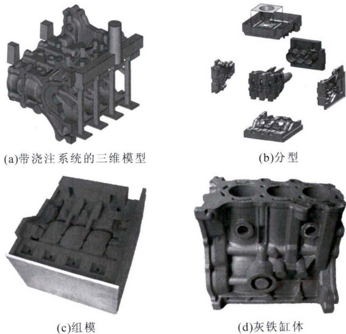
图 8 铸铁缸体制备流程 Fig.8 Preparation process of cast iron cylinder
