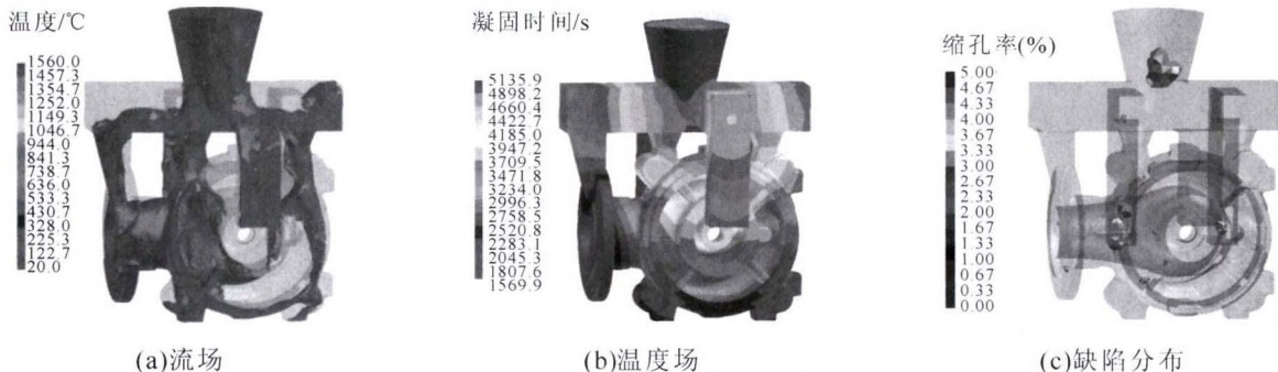
图5 顶注加侧注浇注时铸件模拟结果 Fig.5 Simulation results with top and side pouring system
