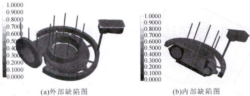
图 8 铸件内部缺陷情况图 Fig.8 Internal defects of castings
