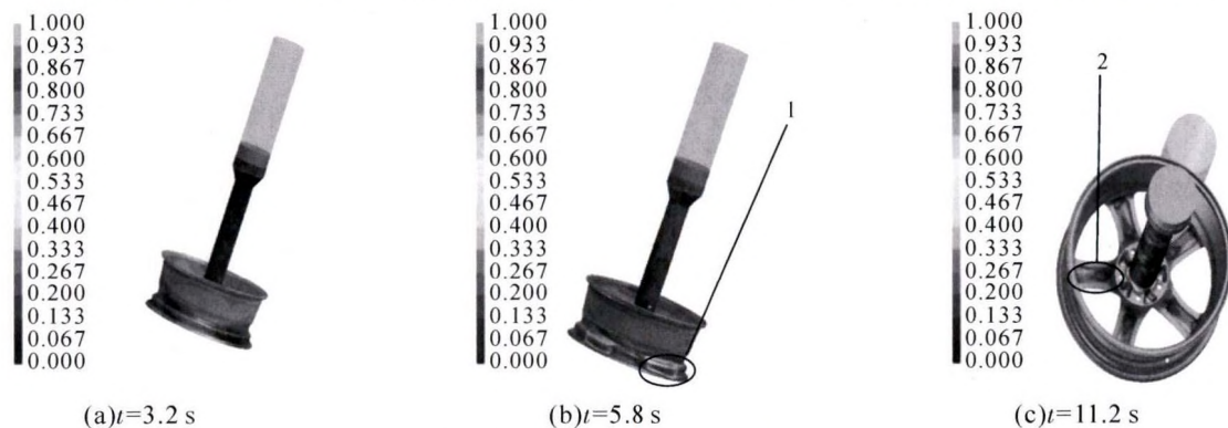
图3 不同时间下的凝固过程固相率 Fig.3 Solid phase ratio during solidification at different times
