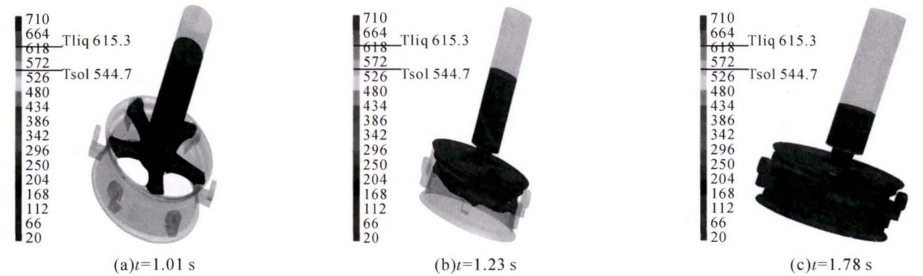
图 6 优化后不同浇注时间的充型温度场 Fig.6 Filling temperature field with different pouring time after optimization
