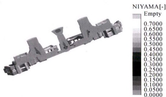
图7 Niyama(补缩能力分析)判据 Fig.7 Niyama criterion
