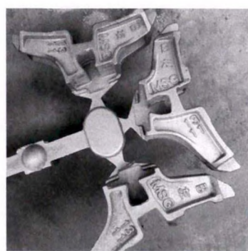
图9 铸件带浇注系统实物图 Fig.9 Castings and riser and gate system
