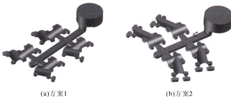
图2 两种不同的浇注系统设计 Fig.2 Two type of designs of different gating system structures
