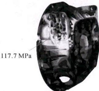
图8 原壳体应力集中分析 Fig.8 Stress concentration analysis of the original housing
