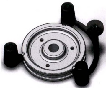
图3 轮缘处进铁液方案 Fig.3 Molten iron feeding scheme at the rim
