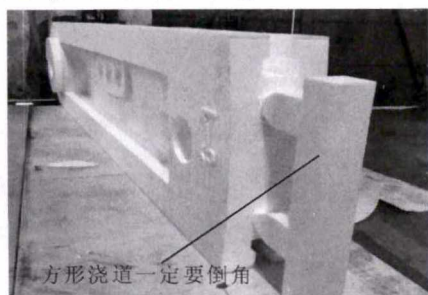
图 14 端面阶梯浇注系统 Fig.14 Stepped pouring system at end face of the casting
