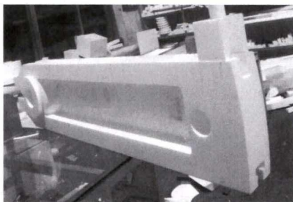
图 26 粘好浇注系统的泡沫模 Fig.26 Foam pattern adhered with pouring system
