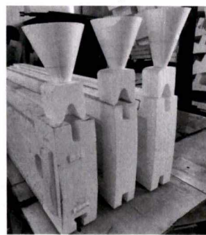
图 39 浇注系统尺寸适当调整 Fig.39 Size of pouring system properly adjusted
