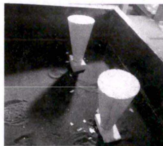
图 34 加砂埋型处理浇口杯 Fig.34 Filling sand to fix foam pattern and pouring cup patterns
