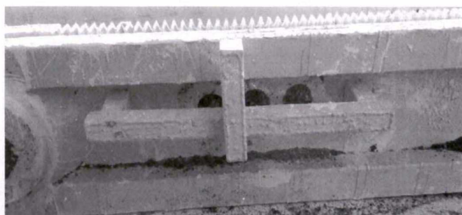
图 5 6 型曲柄原工艺浇注系统 Fig.5 Original pouring system of Type 6 crank casting
