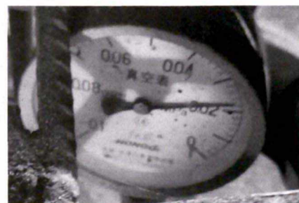
图 32 浇注时负压维持在 0.02 MPa Fig.32 Maintain negative pressure at 0.01 MPa
