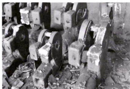
图 33 铸件降温过程中, 涂料壳自行剥落 Fig.33 Coating shells peel off during cooling
