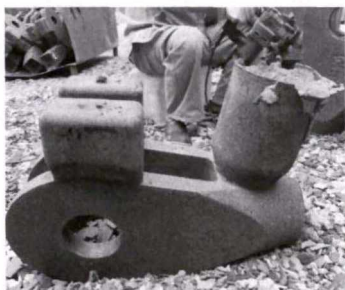
图 34 涂料壳基本自行脱落 Fig.34 Coating shells peel off themselves during cooling
