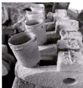
图 23 焙烧后的模型空壳 Fig.23 High temperature sintered shell molds
