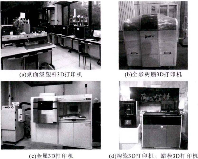
图 2 实验室现有 3D 打印机分类 Fig.2 Classification of existing 3D printers in the laboratory
