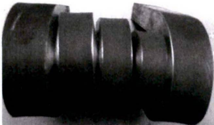
图 2 S355J2W(H)不同厚度钢板冷弯试验 Fig.2 Cold bending test of S355J2W(H) steel with different thickness
