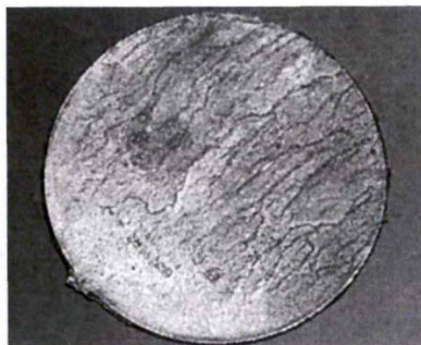
图 5 铸件表面的水痕类缺陷 Fig.5 Watermark defects on the casting surface
