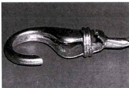
图8 铸件不完整 Fig.8 Incomplete casting
