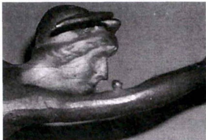
图 3 铸件表面的球状缺陷 Fig.3 Spherical defects on the casting surface
