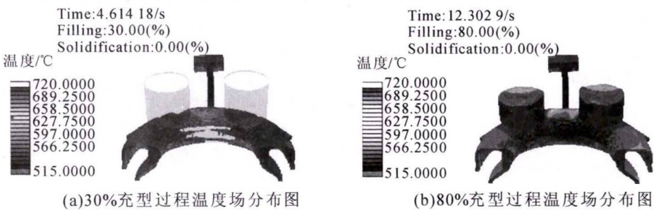
图 5 半圆环板充型过程温度场分布图 Fig.5 Temperature Field Distribution of During Filling
