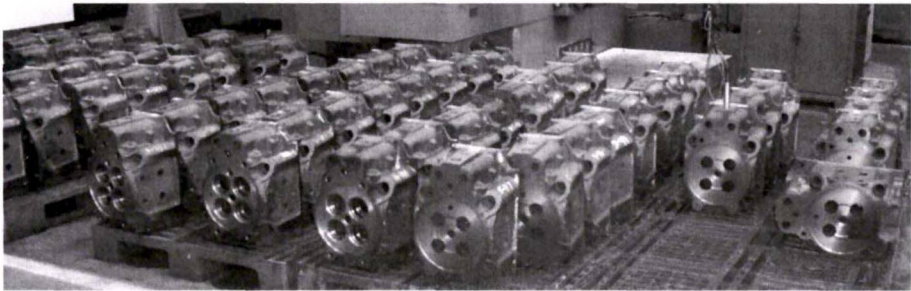
图 3 批量生产的缸盖零件实物 Fig.3 Machined cylinder head of batch production
