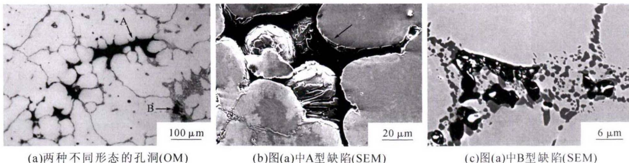
图 8 HK40 合金铸件壁厚中间位置处的缺陷组织 Fig.8 Defective structure in the middle of wall thickness in HK40 alloy casting
