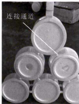
图 33 金字塔组合 Fig.33 Pyramid shaped cluster of lost foam patterns
