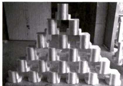
图 28 小件 6 层叠罗汉 Fig.28 A cluster with 6 layer of lost foam patterns
