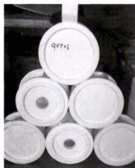
图 32 金字塔组合 Fig.32 Pyramid shaped cluster of lost foam patterns
