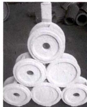
图 34 整体浸涂 Fig.34 Whole cluster is in dipping coating
