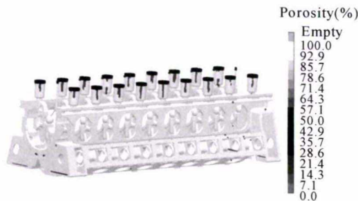
图 10 机身凝固过程模拟图 Fig.10 Simulation of cylinder block solidification process
