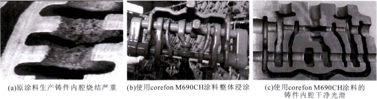
图 7 corefon M690CH 涂料浸涂效果 Fig.7 The corefon M690CH coating dip coating effect
