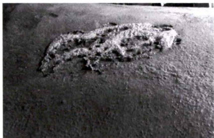
图6 铜合金螺旋桨的夹砂缺陷 Fig.6 Scab defects of copper alloy propeller
