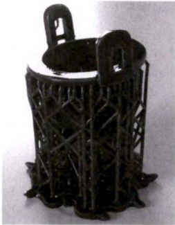
图 6 3D 打印带支撑蜡模 Fig.6 3D printed wax pattern with support
