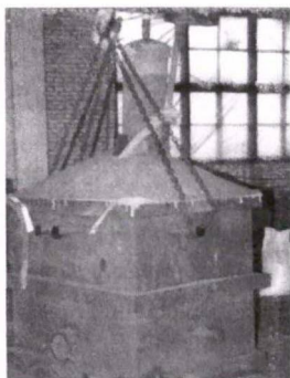
图8 开箱出砂 Fig.8 Open the mold and out of the sand
