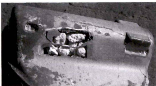
图 1 砂眼 Fig.1 Sand hole defects
