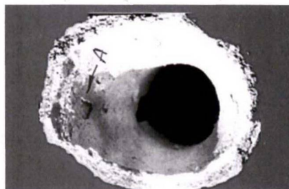
图 7 型壳面层剥落 Fig.7 The Peeling off of shell surface
