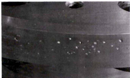
图 2 加工后发现的砂眼 Fig.2 Sand hole defects after cutting process
