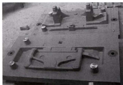
图 15 根据优化的铸件设计,制造的型板 Fig.15 According to the optimized casting design, manufactured the mold plate
