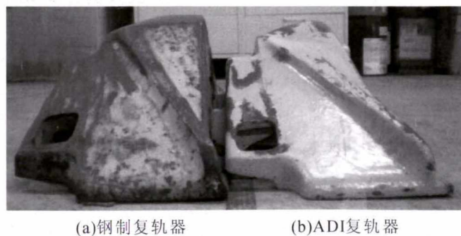
图5 钢制复轨器(左)和 ADI 复轨器(右) Fig.5 Steel retracer (left) and ADI retracer (right)
