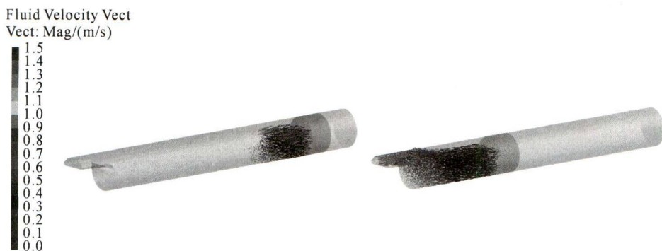
图8 正交试验表中6#工艺条件下压射室内金属液流场分布状态 Fig.8 Flow field of molten metal in the injection chamber under No. 6 orthogonal test
