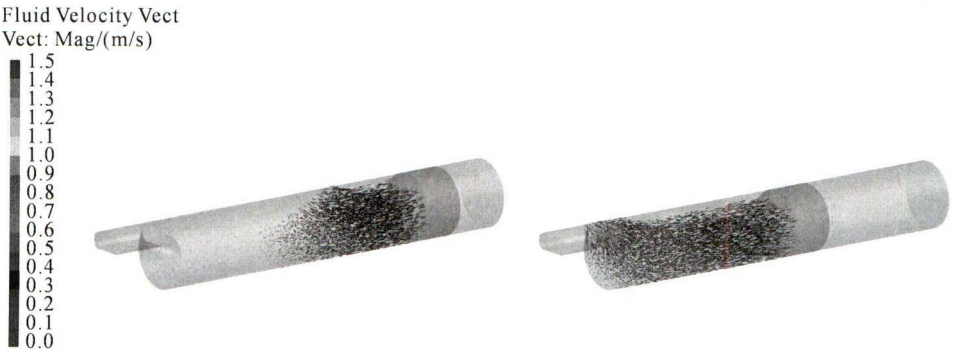
图 6 正交试验表中 5# 工艺条件下压射室内金属液流场分布状态 Fig.6 Flow field of molten metal in the injection chamber under No. 5 orthogonal test
