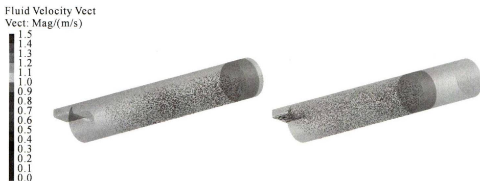
图10 正交试验表中14#工艺条件下压射室内金属液流场分布状态 Fig.10 Flow field of molten metal in the injection chamber under No. 14 orthogonal test
