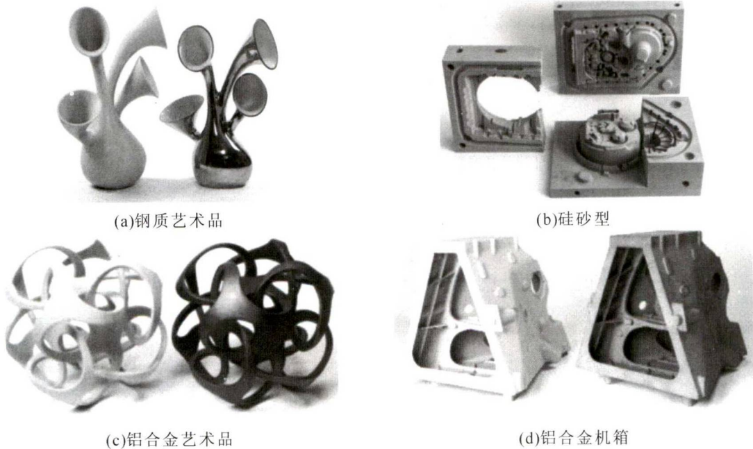
图 2 3D 打印的零件和砂型 Fig.2 3D printed parts and sand molds
