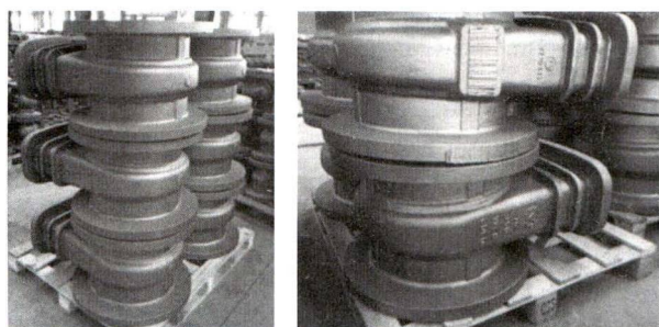
图9 新工艺试制的经热处理抛丸后的铸件 Fig.9 Trial-produced, heat treated and shot blasted valve body with new casting process
