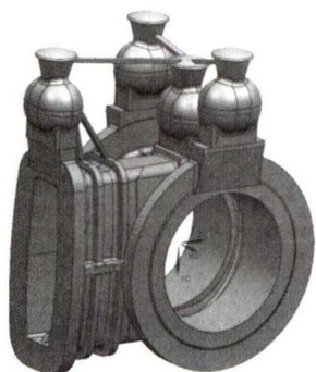
图5 阀体浇冒口系统示意图 Fig.5 Schematic gating and riser system for the valve body casting
