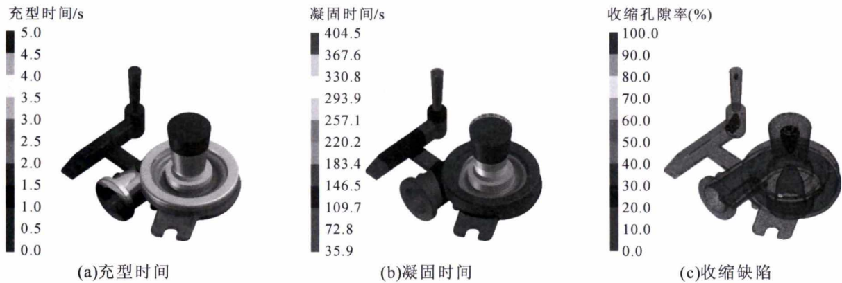
图 6 铸造工艺二次优化仿真结果 Fig.6 Simulation result of secondary optimized casting process
