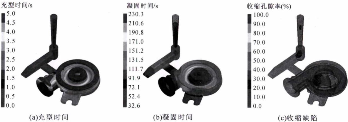
图4 铸造工艺仿真结果 Fig.4 Simulation result of casting process
