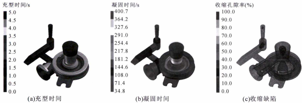
图 5 铸造工艺初步优化仿真结果 Fig.5 Simulation result of initial optimized casting process
