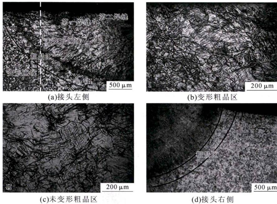
图 7 Microstructure of the ITW welds of NB steel<sup>[22]</sup>
