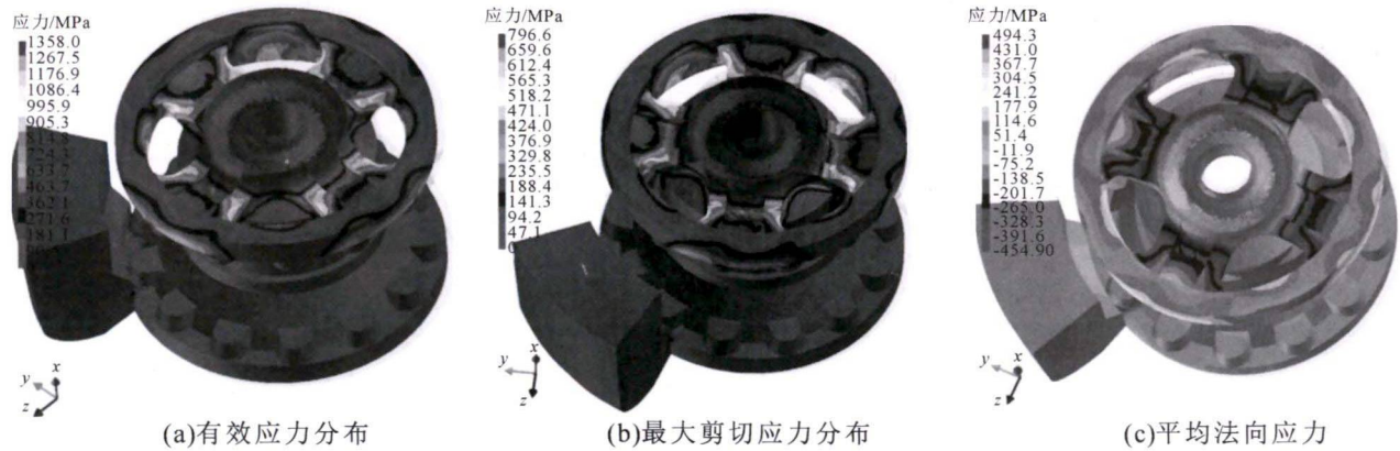
图6 应力分布模拟预测 Fig.6 Stress distribution simulation prediction
