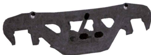
图9 工艺优化铸件凝固过程数值模拟结果 Fig.9 Numerical simulation results after solidification process optimization
