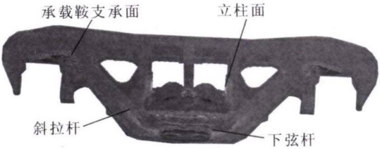
图 4 侧架最后凝固区域 Fig.4 The final solidification area of the side frame
