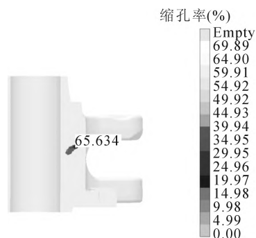
图3 基于MAGMA模拟浇注温度为1380℃挂钩缩孔缺陷 Fig.3 MAGMA simulation for hook shrinkage defects with 1380℃ pouring temperatures
