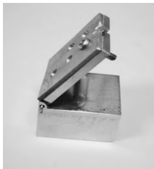
图3 T-EBSD样品台实物 Fig.3 The T-EBSD sample station
